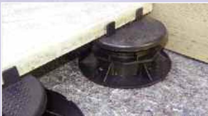
Mini Bases are designed for use with the ASP range. They have a 150mm diameter base which means both base and head can be butted up against the upstand or parapet wall without a gap between the slab and the wall.
