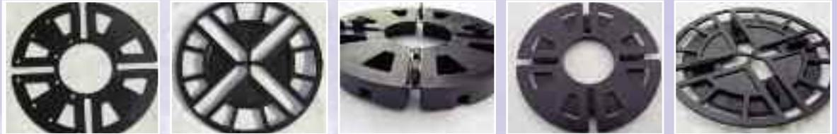
Shims are available 1mm, 2mm and 3mm thick. They are loose fitted and held in place by the positioning lugs. The 3mm thick shim has a slightly different shape to the 1mm and 2mm shims, but all three are suitable for all of the fixed height supports. The shims will overhang the rubber ring slightly, but this is no issue. The weight of the slab will ensure that the whole system is held in place properly.
