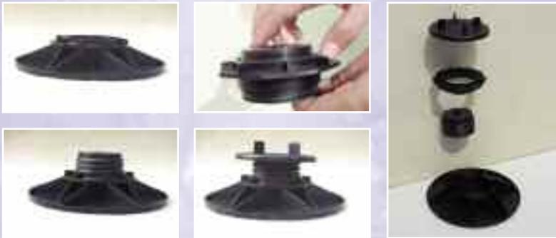
The base plate is a solid, round base measuring 200mm in diameter. In the centre of the base is a round collar in which the stem and nut will sit. It is designed so that the weight will pass down the stem and onto the outside of the collar, and then pass down along the diagonal arms spreading out across the face of the base plate.
