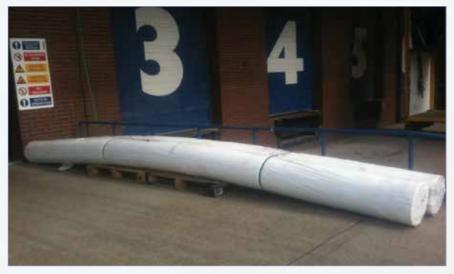
These super-jumbo rolls are designed for use for very large projects, such as road construction, reservoirs and landfills. Using very wide rolls reduces the number of joints between individual rolls. This cuts down on labour by having less individual rolls to stitch together, and also makes the whole fabric layer stronger by having less weak points at the joints.
