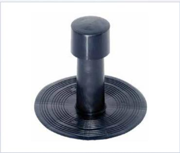
The top of the tube or flue has three holes to allow the vapour to escape into the atmosphere. It is covered by a hood or cap which overlaps the internal holes, preventing rainwater entering the system but still allowing the passage of vapour.
