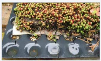
By designing an "egg-box" profile, blockages are prevented and a greater amount of water can pass along the membrane. This profile also allows very easy sealing of the membrane, as multiple sheets can be "clipped into place" by overlapping the cups and sealing the joints with adhesive tape.
