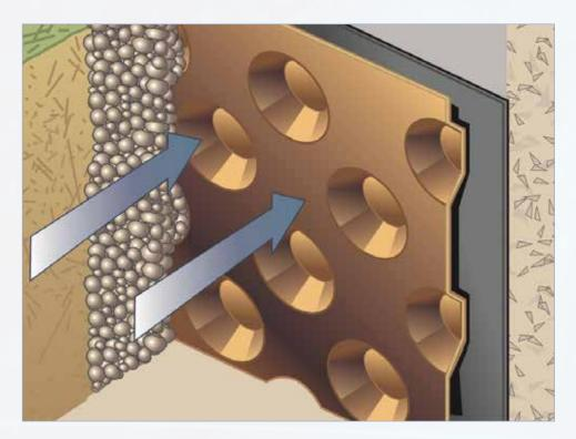
The 8mm high cups create an air gap between the structure and the earth backfill, helping to ventilate it effectively.
