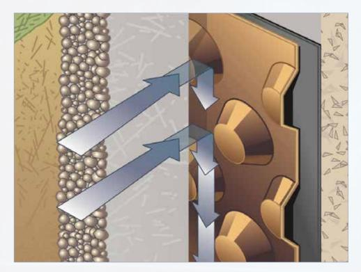
This gives additional protection to the membrane and also helps to filter out particles whilst allowing the water to pass through the fabric and into the air gap drainage chamber.
