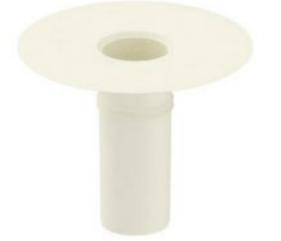
**Function:** Circular PVC drain connector designed to be welded to prefabricated synthetic PVC waterproofing membranes to connect to downpipe rainwater drains. They have a smooth flange to improve welding to the membrane; they have two rings on the outside of the shank which acts as drain trap to help seal the gap between the drainage outlet itself and the rainwater drain. The shank is slightly tapered to help installation into the drainpipe.
