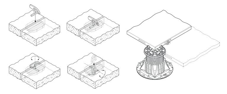
To remove the Ventus Uplift Bracket, use a screwdriver to slide between the gaps in the tiles to swing the underside up and grab with fingers. Twist the central column again to release the bar from the tile cuts.
