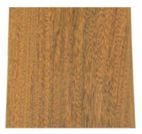
It is a very widely used wood in the decking industry and can be used for small, medium or large floors, subjected to low or high levels of foot traffic, in private residential and commercial projects with a variety of different fixing details. It can also be used for cladding.
