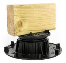
Place timber or composite joist onto headpiece between the positioning lugs so it is suspended on top of the pedestal. There is no need to mechanically fix the joists to the pedestals.
