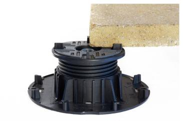
Slabs / tiles are loose laid onto headpieces between four integrated lugs to position and separate them and provide 4mm gap for drainage. The Yellow Key is used to adjust the height of the pedestal after the full system has been installed without having to lift the slab / tile https://www.youtube.com/watch?v=Ky8WMTR67xQ.
