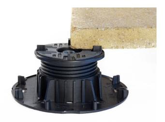
Slabs / tiles are loose laid onto headpieces between four integrated lugs to position and separate them and provide 4mm gap for drainage. The Key is used to adjust the height of the pedestal after the full system has been installed without having to lift the slab / tile <a href="How to use">How to use "The Key"</a> to adjust the Mega-Balance Pedestal - YouTube.
