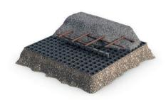
Protecto-Drain 8 assumes the function of previously used lean concrete, offering climate-independent working and eliminating waiting times for concrete to harden. The dimpled membranes are easily rolled out on a level and stable surface. During installation, overlap the membranes lengthwise and crosswise by 20 cm to ensure proper coverage. Protecto-Drain 8 provides protection against rising moisture and prevents downward flow of cement paste.
