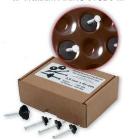
The steel fixing studs and mounting knobs can be used to efficiently install dimpled sheets and fasten them to concrete and masonry. The mounting knobs prevent the dimpled sheets from tearing the membrane and help to seal the fixing hole.
