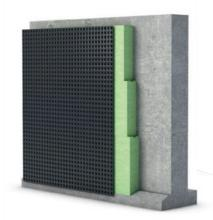
Protecto-Drain 8 is laid directly on a pressure-resistant sealing (waterproof concrete or perimeter insulation) with the dimples facing the structure. The membranes must be laid higher than, for example, the perimeter insulation, and fixed there temporarily. Bevel the perimeter insulation at the upper edge. The flat overlapping margin allows a fitting connection. After backfilling, the dimpled membrane is cut to the correct length and completed with the Wallbarn EDGING PROFILE.
