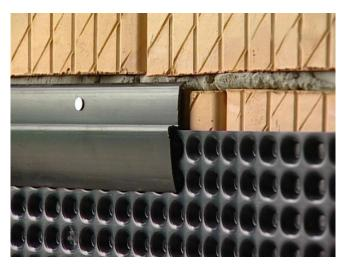
2. Wallbarn EDGING PROFILE made of plastic in black. An edge profile is used as the top finishing element on dimpled and drainage membranes. It reliably prevents stones and soil from falling behind the dimpled sheet. The profile is equipped with pre-punched holes, so that it can be securely fastened to themasonry. The plastic profile can be used in a non-visible area.
