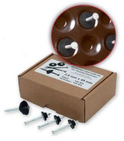
The steel fixing studs and mounting knobs can be used to efficiently install dimpled sheets and fasten them to concrete and masonry. The mounting knobs prevent the dimpled sheets from tearing the membrane and help to seal the fixing hole.
