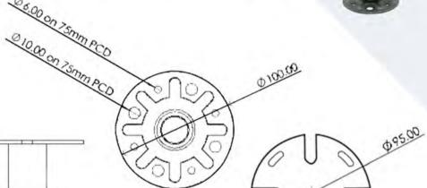
MetalPad EX comes as a flat headed pedestal as standard. They will support paving and decking systems for pedestrian spaces including balconies, roofs, podiums and terraces. A number of headpiece options are available which click quickly and easily into place. Each
